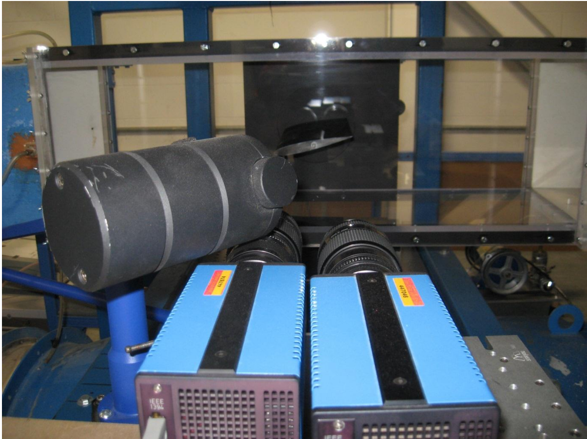
Figure 22: Camera set-up (left camera for leading edge zoom view, right camera for entire airfoil view)
